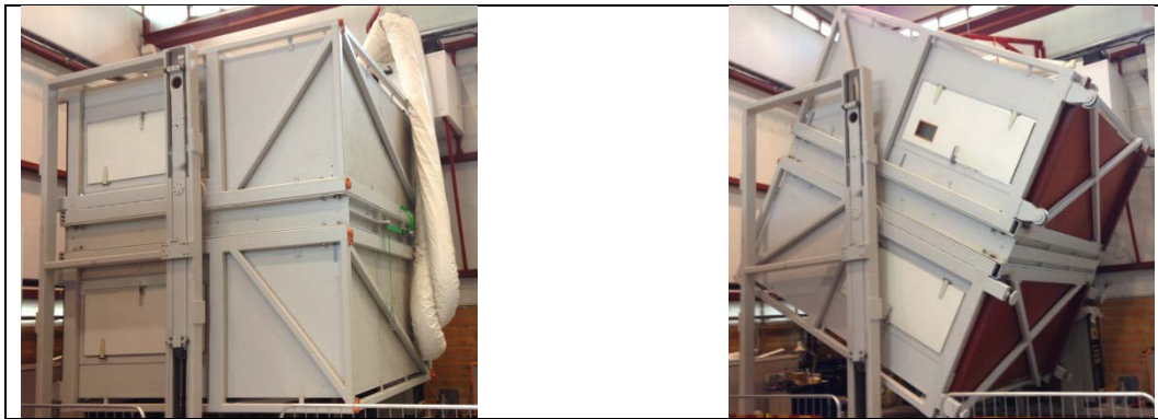
Figure 3. The rotatable Hot-Box test facility. To the left, the test section is positioned as a floor (cold room below the test section). To the right, the angle of inclination of the test section is 30°.
