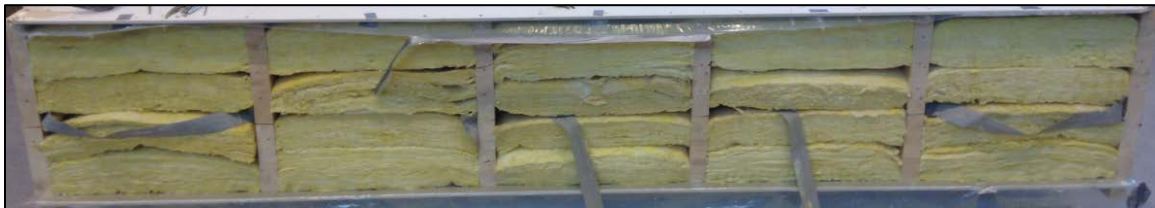
Figure 8. Air gaps in transition zones between the layers of insulation and between the insulation and the wood frame.
