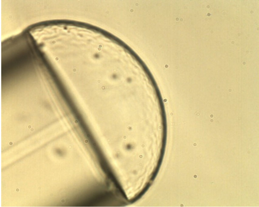
Figure 3: Optical micrograph of hemispherical hydrogel, covalently attached to the end of an optical fiber. Reproduced from [2] with permission. The diameter of the fiber is 125\ \mu\text{m} , while L_g is typically 50\ \mu\text{m} .
