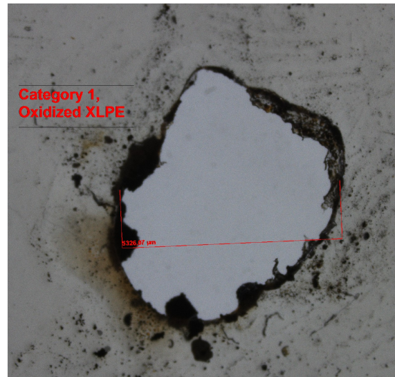
Figure 4.55: Microscope picture of the site of breakdown in a typical category 1 object.
