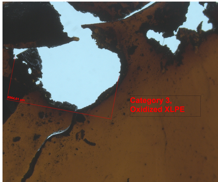
Figure 4.57: Microscope picture of the site of breakdown in a typical category 3 object.
