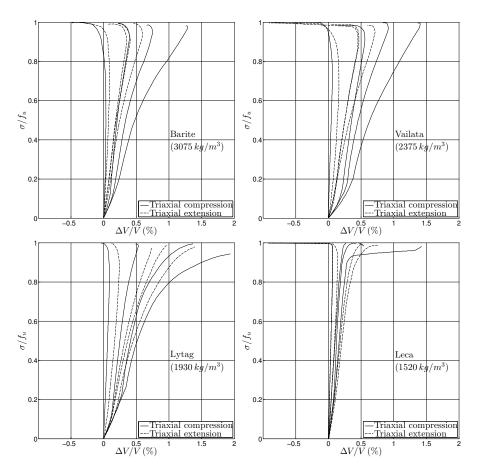
Figure 2: Deformational data presented as the volume variation versus the applied stress normalized by the failure stress.
