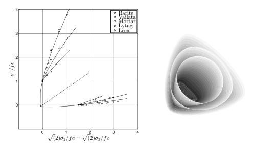
Figure 6: Failure envelopes in the axisymmetric stress plane according to the proposed densitydependent octahedral expressions together with the corresponding complete failure surfaces.
