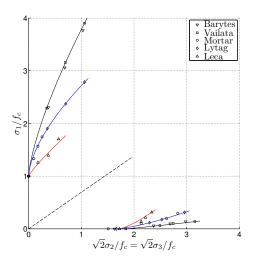
Figure 1: Strength data in the axisymmetric stress plane.
