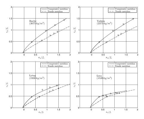
Figure 5: Comparison of strength data to the proposed density-dependent failure criterion.
