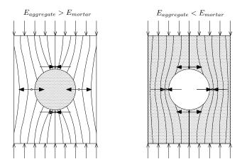
Figure 9: Internal stress transfer in concrete under a compressive load for either: a stiffer and stronger aggregate embedded in a softer and weaker mortar; or a softer and weaker aggregate embedded in a stronger and stiffer mortar [37].
