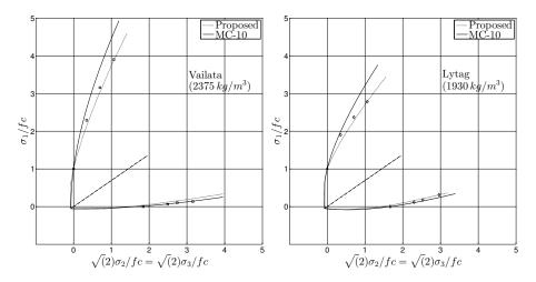
Figure 7: The failure criterion in MC-10 and the proposed density-dependent criterion compared to the strength data from the ENEL tests.
