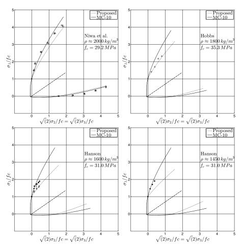
Figure 8: Strength data in the axisymmetric stress plane according to tests
