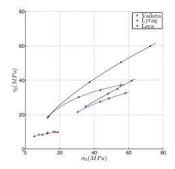
Figure 4: Failure envelopes in the octahedral stress plane.
