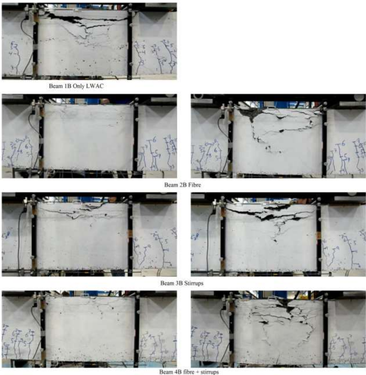
Fig. 8: Failure zone in beam at peak load (left) and at 0.9P_{spall} (right)
