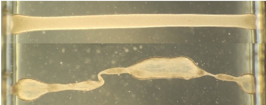
Figure 5.23: Shows a 4 wt.% Na-Fh drop making a bridge in a 500 V/mm field after 10 seconds(top) and 3 min(bottom). Initial drop radius \sim 0.775 mm.
