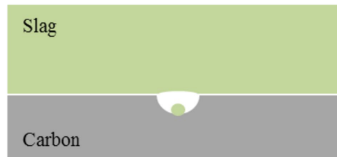
e) Slag micro-droplet reduction and and Mn evaporation
