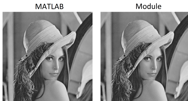
Figure 4.11: The resulting inverse DWT of the output of the wavelet transform module.
