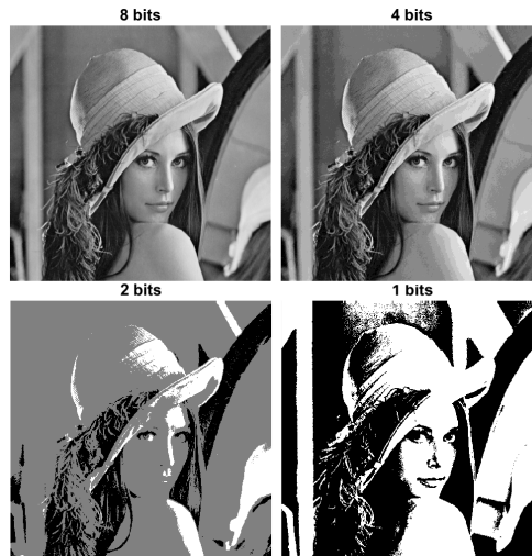
Figure 2.16: Different bit depths for an grayscale image.
