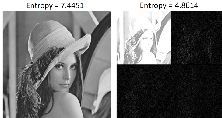
Figure 2.38: The entropy difference of an image and its 1 level DWT decomposition.
