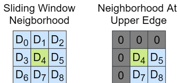
Figure 2.47: The neighborhood of samples formed by the sliding window. Samples outside the code block is set to 0.
