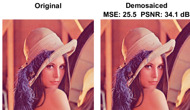
Figure 2.12: Original image vs image transformed to Bayer pattern and then demosaiced.
