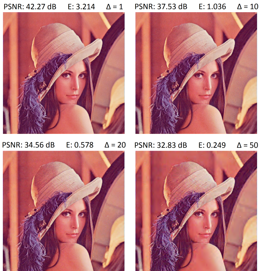
Figure 4.15: Reconstructed image after inverse wavelet transformation and dequantization with R=0.1 .
