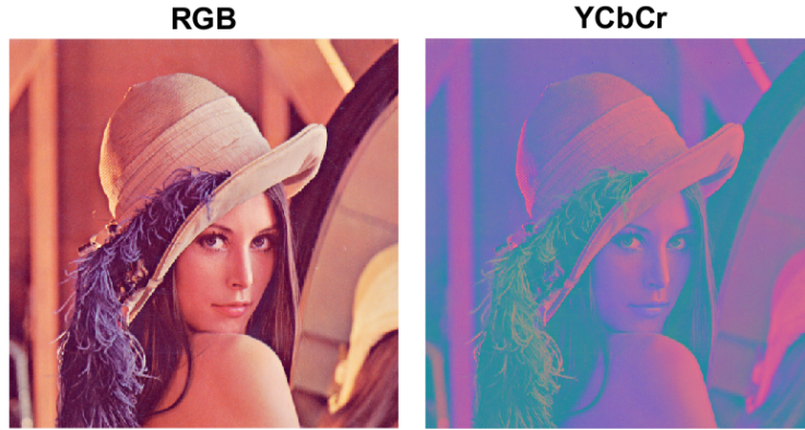
Figure 2.19: Conversion from the RGB color space to YCbCr using irreversible color transform.
