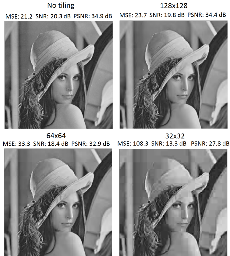
Figure 2.5: The effects of tiling on the compressed image.
