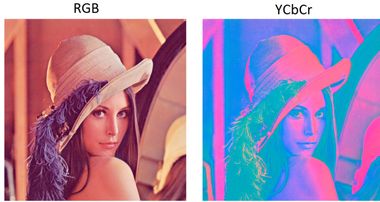
Figure 2.18: Conversion from the RGB color space to YCbCr using the reversible color transform.
