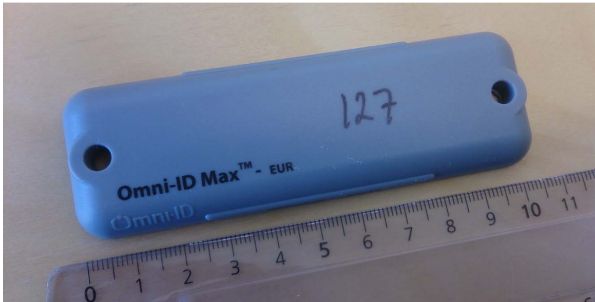
Figure 11: RFID tags that were used were of make and type Omni-ID Max : rectangular, flat, hard plastic tags with a screw hole in each end.
