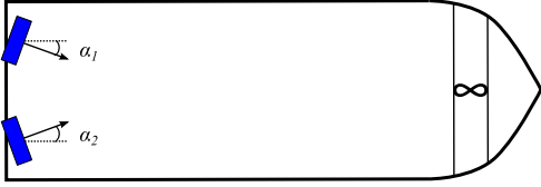
Fig. 4. Biasing of main thrusters placed at the stern
