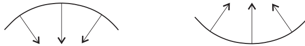
Figure 2.11: Qualitative sketch of the surface tension direction depending on the shape of the surface.
