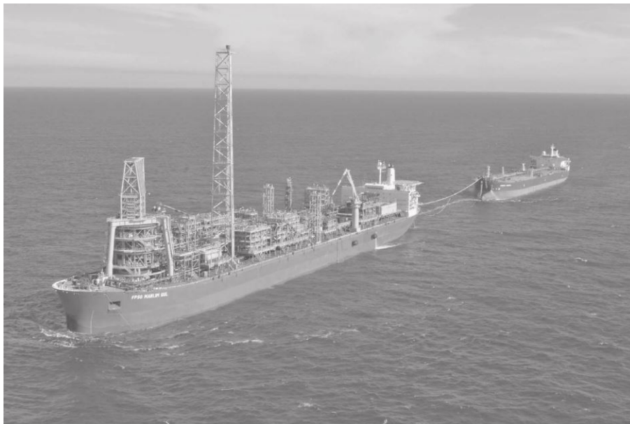
Figure 2.1: Tandem offloading configuration between a turret moored floating, production, storage and offloading (FPSO) and a shuttle tanker (Paik, 2007)
