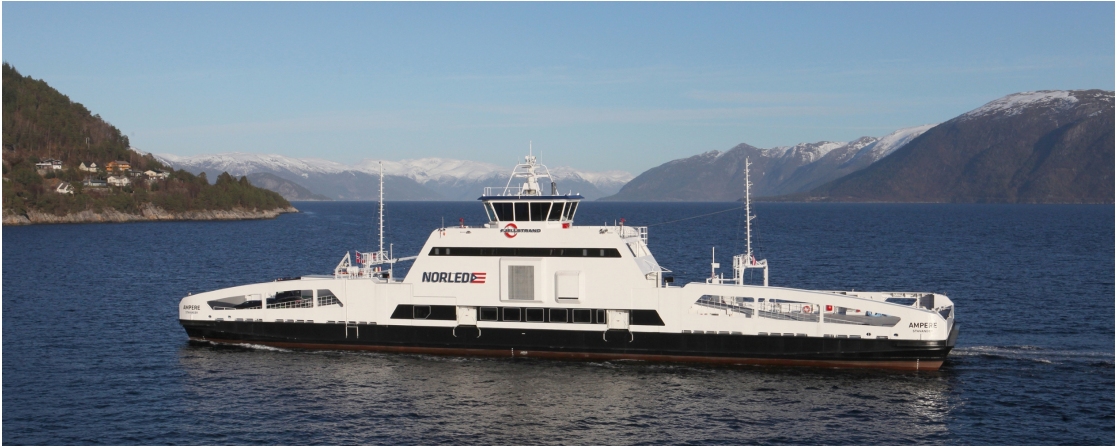
Figure 1.2: The battery-powered ferry Ampere . © 2015 DNV GL.
