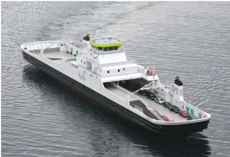
(b) The car ferry Oppedal , a monohull. The ferry operates the route Lavik–Oppedal, and takes 120 PCEs and 350 passengers. © 2017 Skipsrevyen.
