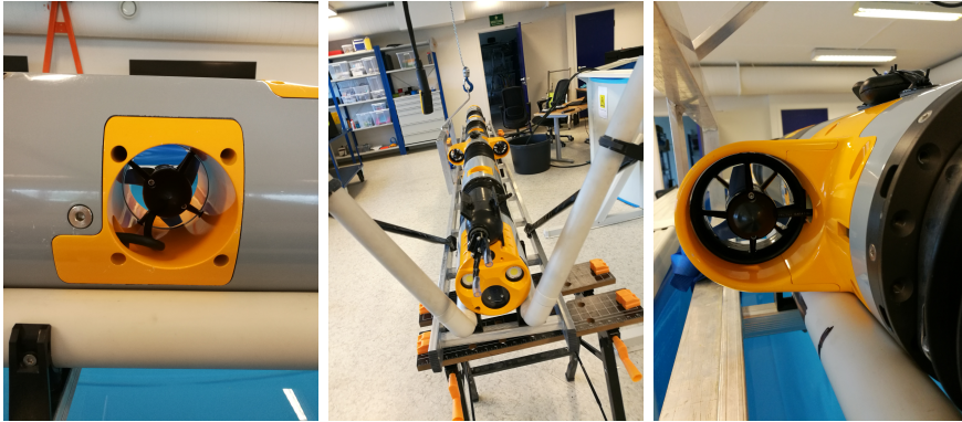
(a) Tunnel thruster (b) The Underwater Snake Robot with Thrusters (c) Main propeller
