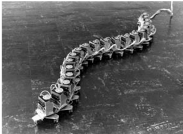
Figure 2.3: The snake robot ACM III, which was the world's first snake robot developed by professor Shigeo Hirose in 1972. From Hirose and Yamada (2009)
