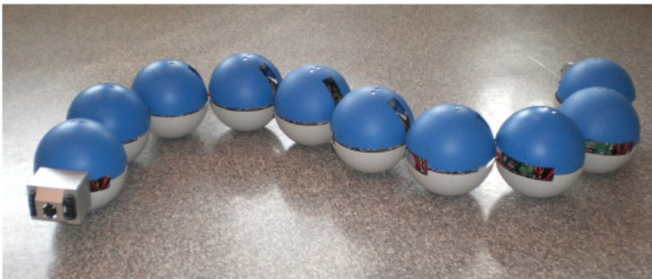
Figure 2.6: The snake robot Kulko, found in Liljebäck et al. (2012b)
