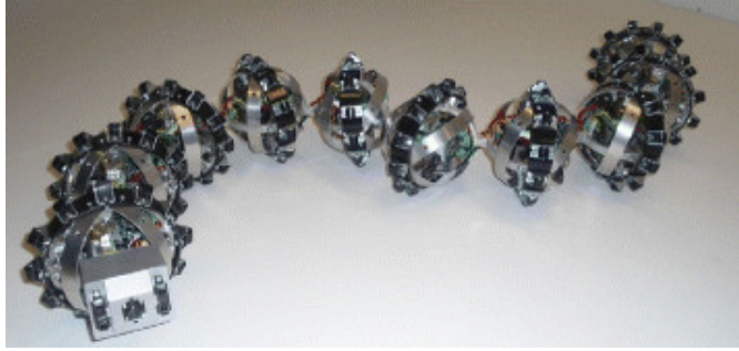
Figure 2.5: The snake robot Wheeko from Liljebäck et al. (2012a)
