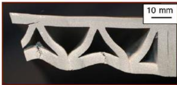
(b) Panel center failure
