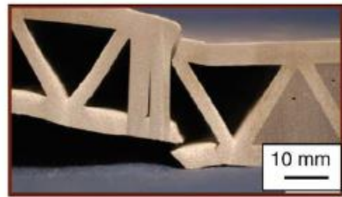
(c) Panel edge failure
