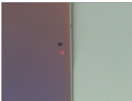
Figure 4.4: After attenuation the laser spot can be imaged on the substrate surface by a CCD camera, here in the vicinity of a \text{MgF}_2 coating edge and a micrometer sized dust particle on the surface. The image width is 400 \mu\text{m} , and the focused laser spot has a full width at half maximum of approximately 5 \mu\text{m} . Due to the 45^\circ incidence angle, the surface is in focus only along a vertical stripe down the middle of the image.
