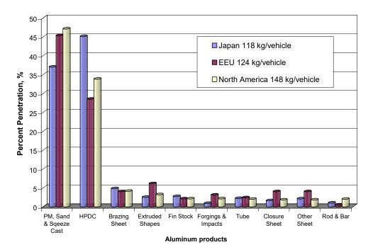
**Fig.3** Light vehicle aluminum content comparison in 2009[13]: EEU: European Economic Union (including Russia in the research); PM: Powder metallurgy, HPDC: High pressure die cast
