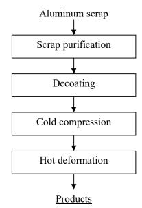
Fig.8 Illustration of solid state recycling
