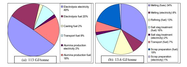
Fig.1 Energy requirements[7] for the production of primary aluminum (a) and secondary aluminum (b)
