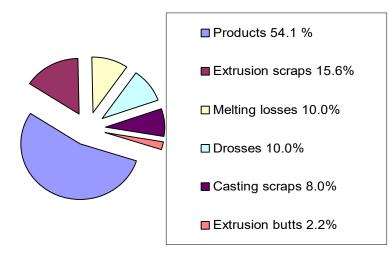
Fig.7 Metal yield in recycling of aluminum turnings by conventional recycling process[25]
