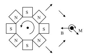
**Fig.5** Illustration of Eddy current separation: Magnet rotor (left) produces a time-dependent magnetic field B inducing eddy currents in a particle (right) resulting in a particle magnetic moment M.
