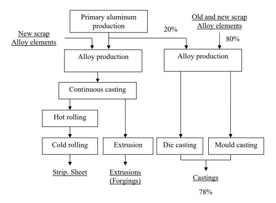
Fig.2 Production scheme for semi-finishes and castings for the automotive sector[12]
