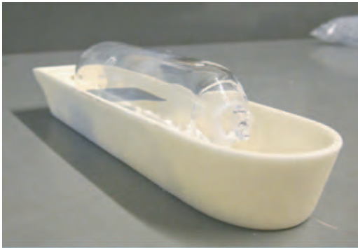
Figure 3.3: Picture of glass ampoule containing a sample, a 25 x 25 mm 2 piece of a wafer.
