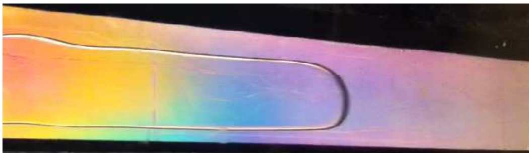
Figure 5.11: Finger made after the clay suspension has been in the cell for 1 hour, and the pistons were pulled with a velocity of 5 mm/s. The experiment is performed using crossed polarizers and a clay suspension of 3,5 wt% Laponite.
