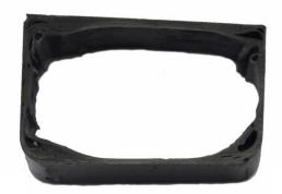
Figure 93: Cross section of bladder moulded sample
