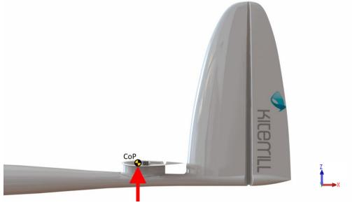
Figure 12: Centre of pressure ahead of the spar
