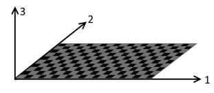
Figure 20: Local coordinate system for a lamina
