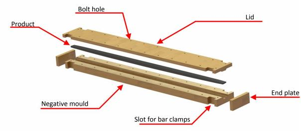
Figure 62: Render of the mould design
