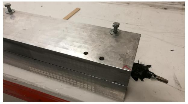
Figure 40: Mould after lay-up with bicycle tube and vale
