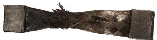
Figure 81: Failure mode for shear samples
