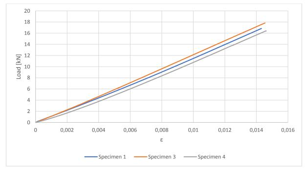
Graph 2: Load vs strain for tension
