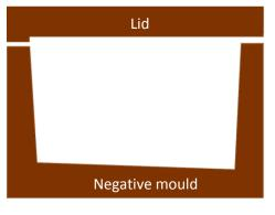
Figure 60: Cross section of the closed mould with slip angle.
