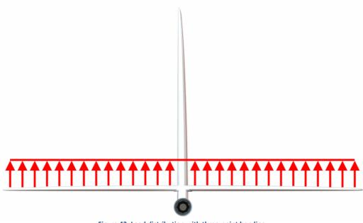
Figure 43: Load distribution with three-point bending.
