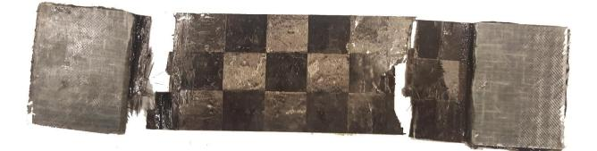
Figure 80: Typical tension specimen failure
