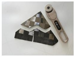
Figure 34: The anti-flaring properties of textreme
