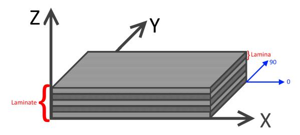
Figure 18: Global coordinate system for the laminate
