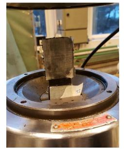
Figure 31: Experimental setup for compression test
