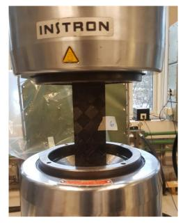
Figure 30: Experimental setup for shear testing
