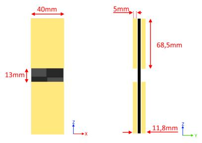
Figure 28: Tab dimensions for the compression specimens
