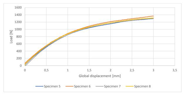
Graph 3: Load vs global displacement for shear samples
