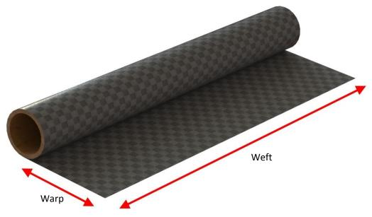
Figure 19: A roll of Textreme (spread tow carbon fiber)
