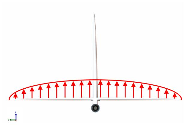
Figure 11: Lift distribution over the horizontal stabilizer
