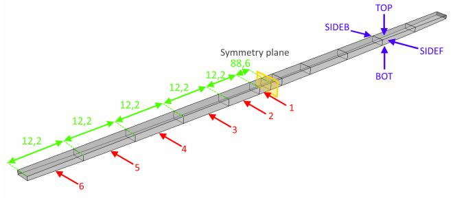
Figure 52: Name notations of the "sets" in Abaqus.
