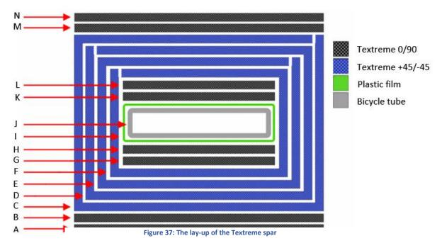
The carbon fiber strips were carefully peeled off the table and placed into the mould. Because the spar is a three-dimensional shape were the cross-sectional perimeter varies along the length, some of the square pieces didn't fit well into the mould. Figure 38 shows that layer square geometry of layer C, D, E and F doesn't fit properly near the ends of the mould. This problem was solved by folding double layer on the top of the spar near the ends. Figure 39 shows the bladder in the mould.
