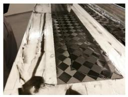
Figure 36: Coloured epoxy distributed on the weave with a spatula
