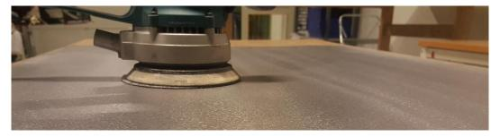
Figure 24: Sanding to remove surface scratches
