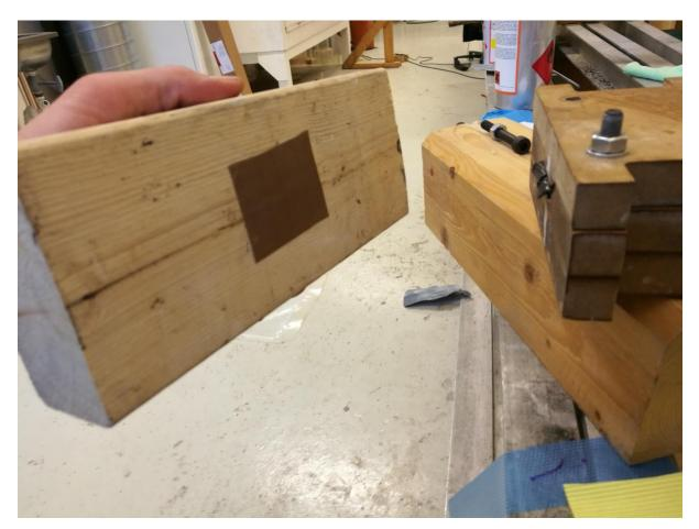
Figure 71: End piece with Teflon tape
