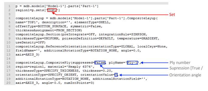
Figure 53: Illustrates the Abaqus macro for importing the properties for a single ply in each set.
