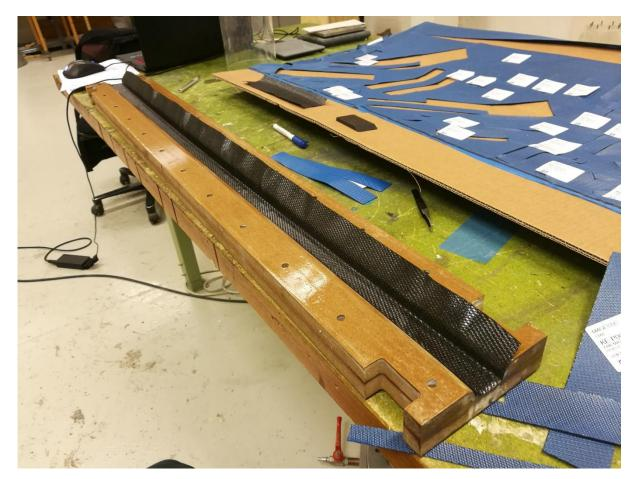
Figure 69: The first ply is placed into the mould
