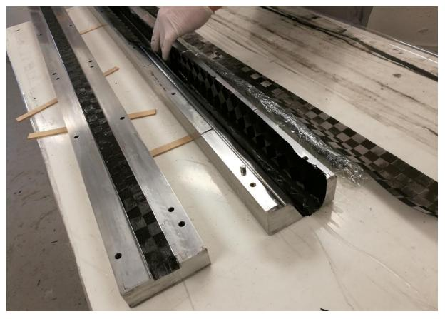
Figure 38: Lay-up process of the carbon fiber
