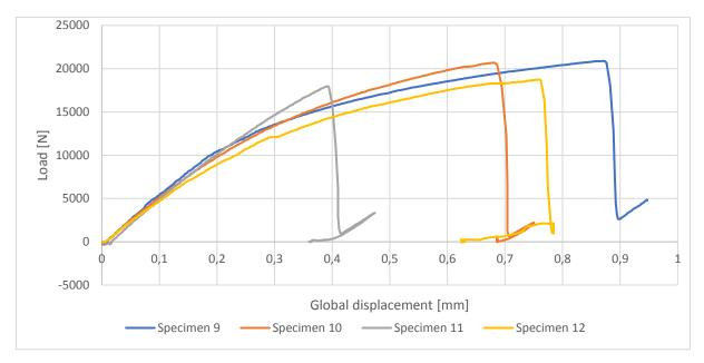
Graph 5: Load vs global displacement for compression samples
