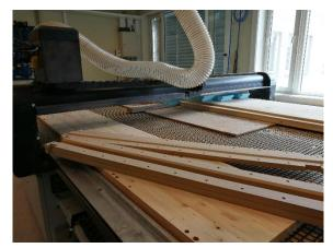
Figure 64: Mould in the milling machine
