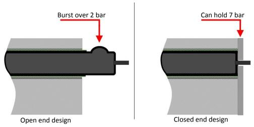
Figure 41: Open vs closed design. The illustration shows how the bicycle tube burst in an open-end mould
