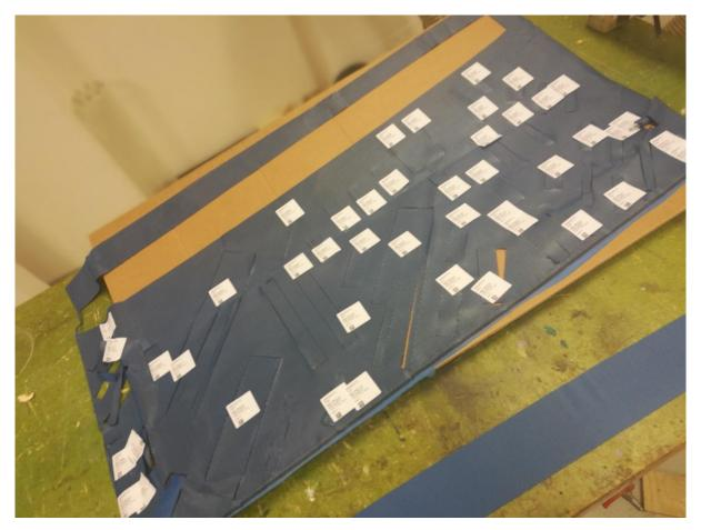
Figure 68: CNC cut plies
