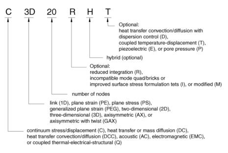
Figure 15: Explanation of the element codes for solid elements (1)
