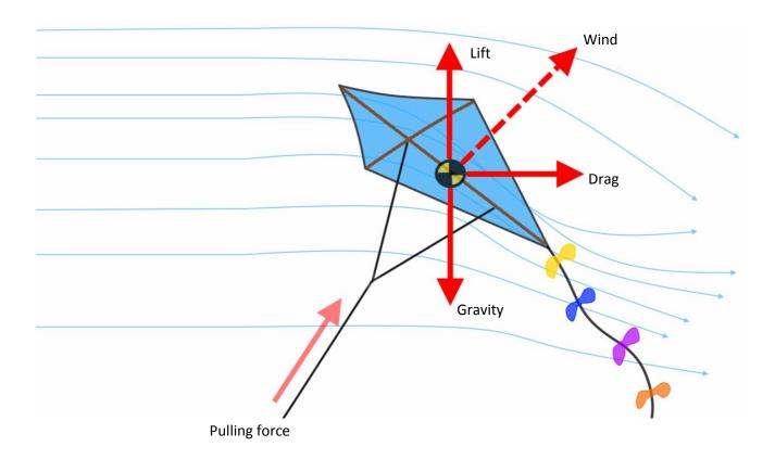
Figure 2: Free-body diagram of a kite
