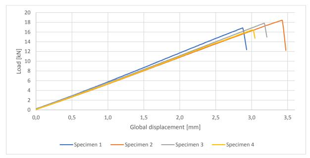
Graph 1: Load vs global displacement for Tension testing
