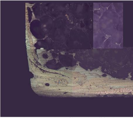
Figure 95 Cross section microscopy of the compression moulded sample
