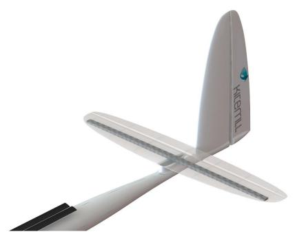
Figure 8: The Horizontal stabilizer spar
