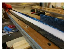
Figure 70: Packing carbon fiber around the core material
