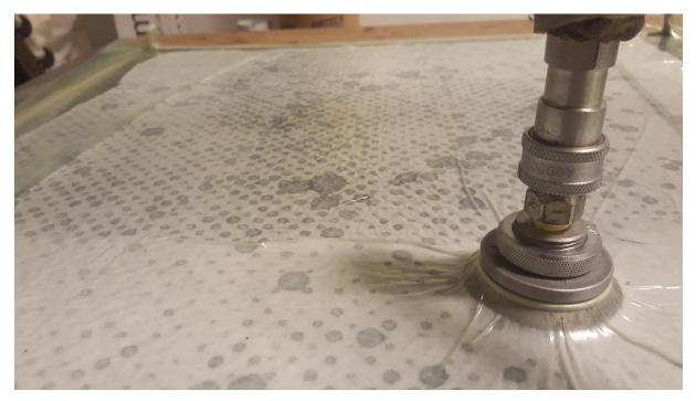
Figure 25: Curing of laminates in room temperature
