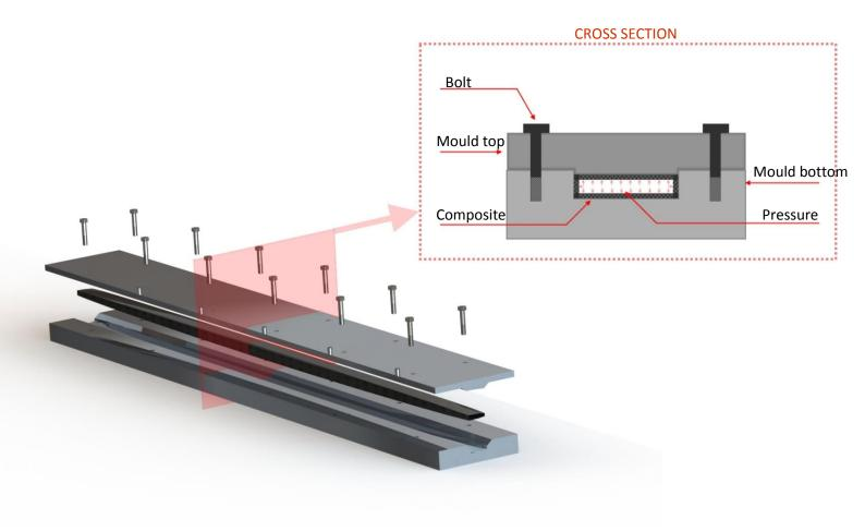
Figure 32: The concept of a closed mould
