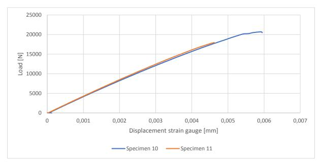
Graph 6: Load vs strain gauge displacement for specimen 10 and 11
