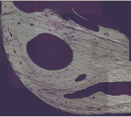
Figure 94: Cross section microscopy of the bladder moulded sample
