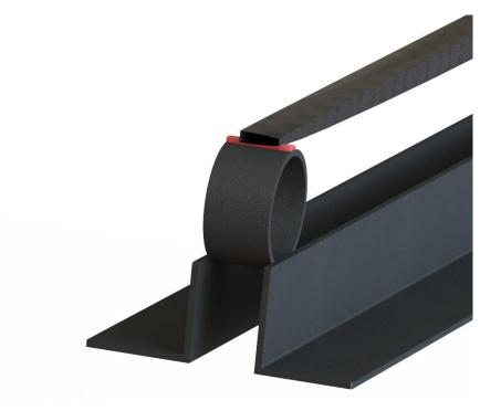
Figure 76: Spacer (Red) between test rig and the spar.
