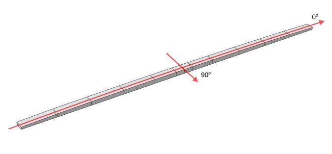
Figure 46: The definition of the material orientation of the Spar
