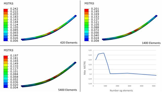
Figure 51: Mesh convergence test
