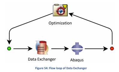
For this flow loop, the limitation of plies was restricted by how many times line 15 - 20 was repeated in the macro file (see Figure 53). In this case the maximum number of plies were set to 20. The data exchanger could suppress the layers by iterating between "True" or "False" in the code, and change the angle of the ply between 0 and 45.
