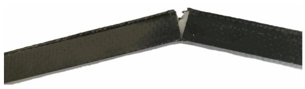
Figure 79: Failure mode of sample 4
