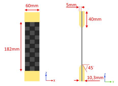
Figure 27: Tab dimensions for tension and shear specimen
