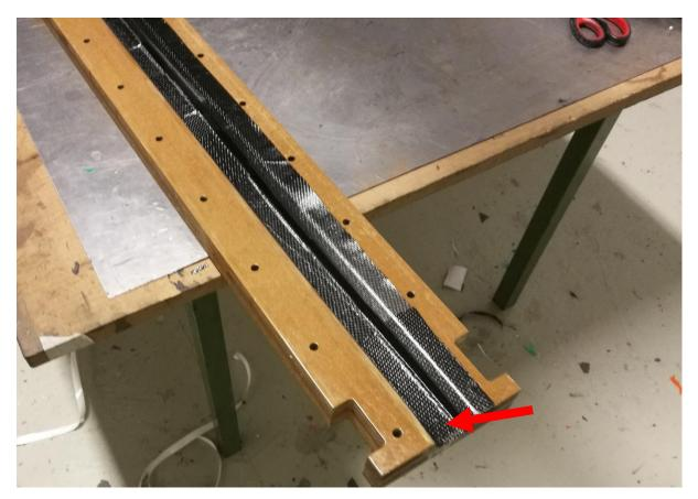
Figure 73: Extra strip of carbon to prevent the carbon from sliding down.
