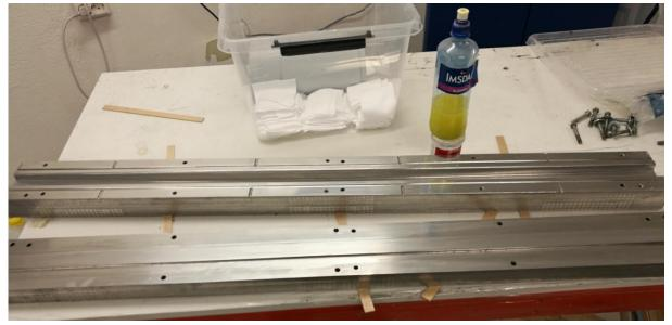
Figure 33: Process of applying release coating
