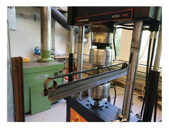
Figure 77: Test setup for testing the spar
