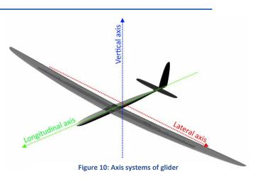
The horizontal stabilizer is used to control the motion of the aircraft in pitch.
