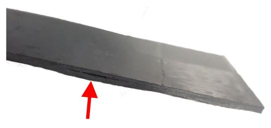
Figure 82: Defect found in one of the compression samples.
