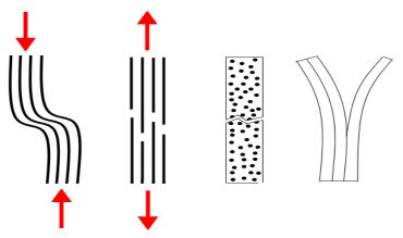
Figure 21: Typical failure modes of composites
