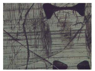
Figure 90: Dry spots in the braiding (5x magnification)
