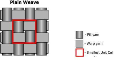
Figure 22: Definition of unit cell (12)
