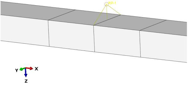
Figure 47: The Kinematic coupling from RP-1 to the center of the spar.
