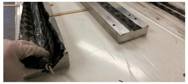
Figure 39: The bladder in the mould
