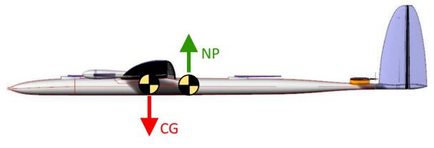
Figure 13: Center of gravity ahead of the neutral point in flying direction.
