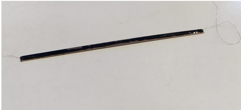
Figure 3.4: MgB 2 wire sample with the reference heater resistance attached with epoxy.
