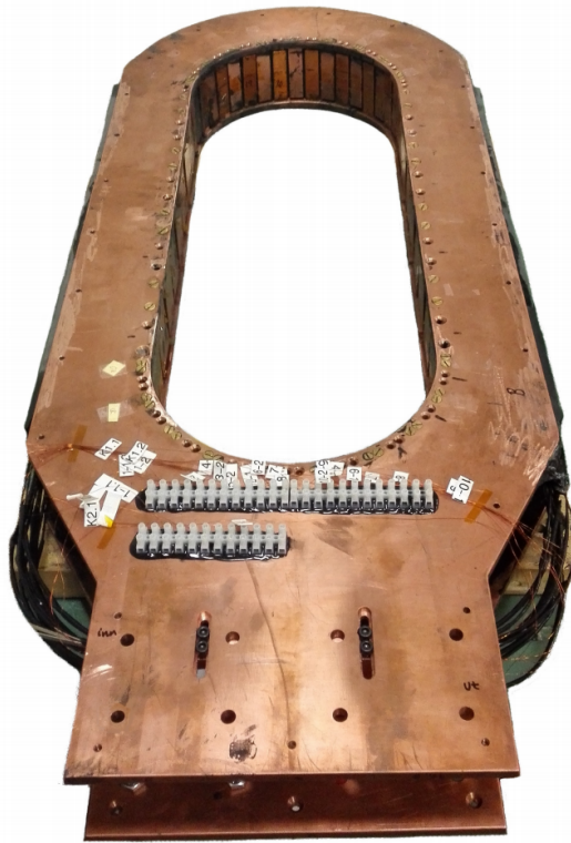
Figure 3.6: Complete field winding with thermal interface [14].
