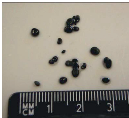
Figure 8: Granules from a UASB reactor treating pulp and paper process wastewater at Norske Skog Saugbrugs, Halden, Norway, were used as inoculum.
