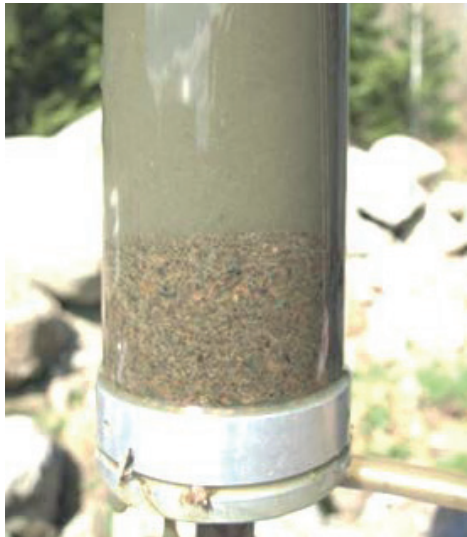
Figure 4: Pig manure sample from the bottom of a storage tank. The particles sediment into a bottom layer leaving a middle layer (upper part of the picture) suitable as high rate UASB AD feed.
