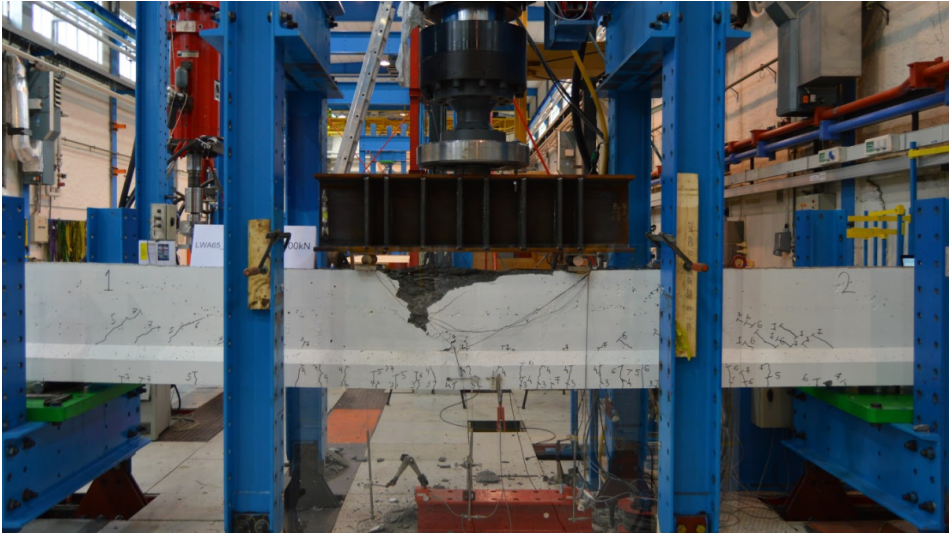
Figure 5.22: Beam 2 - Whole beam, failure
