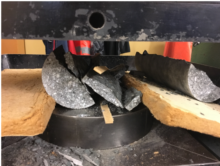
Figure 5.4: Failure of cylinders in tension
