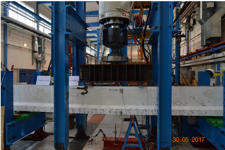
Figure 5.41: Beam 5 - Whole beam, failure
