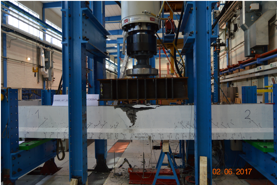
Figure 5.53: Beam 7 - Whole beam, failure
