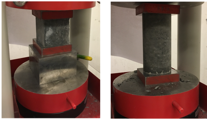
Figure 4.1: Cube and cylinder in the ToniTechnik machine
