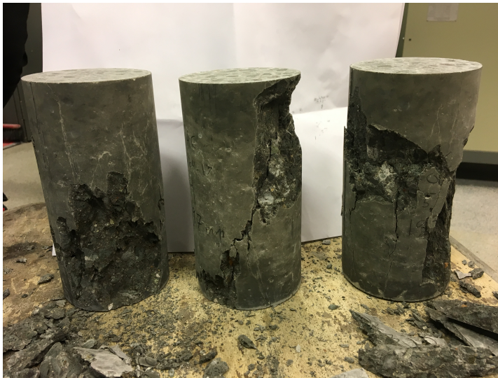
Figure 5.3: Failure of cylinders in compression
