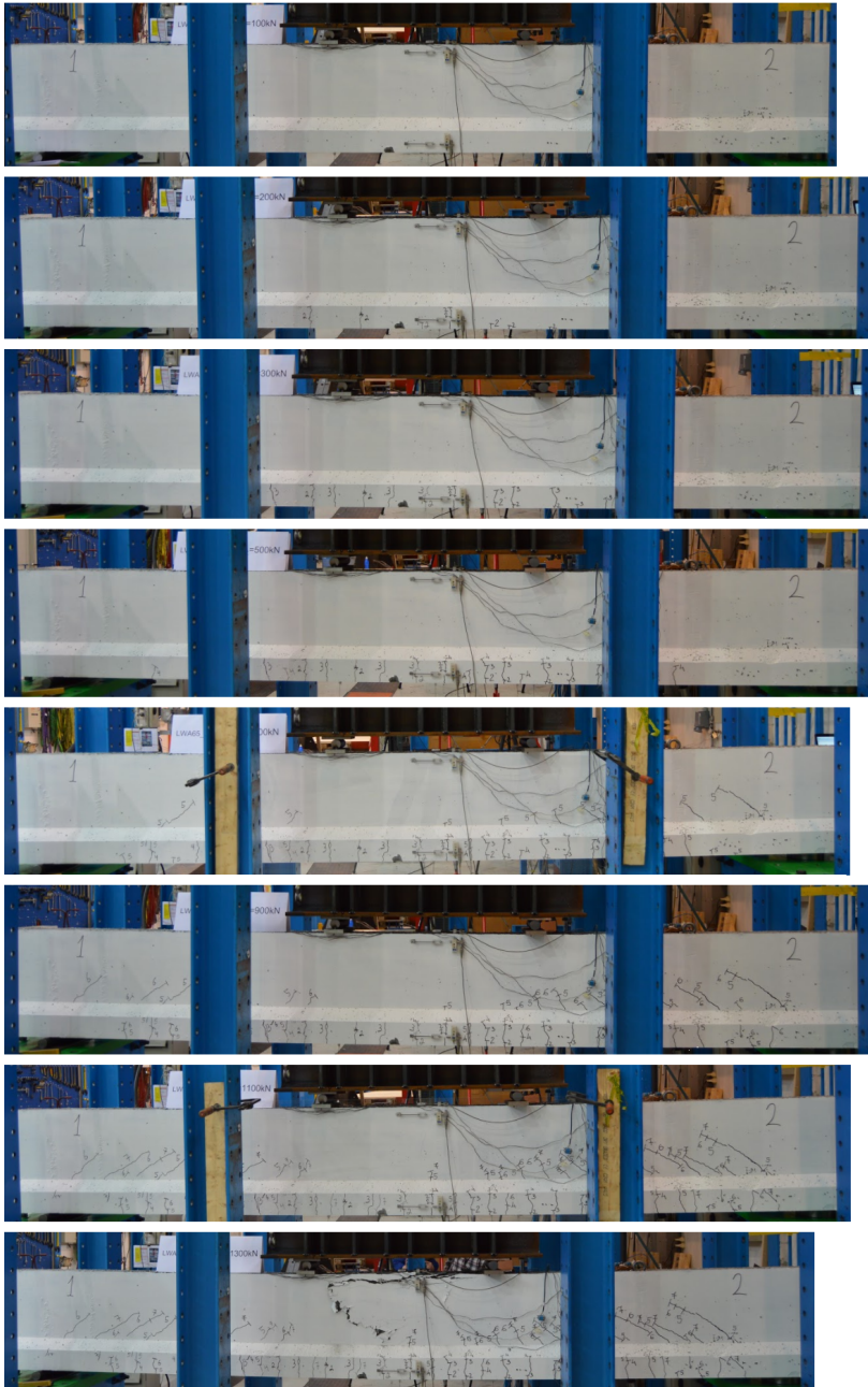
Figure B.4: Beam 3 - Load steps with drawn crack development.
