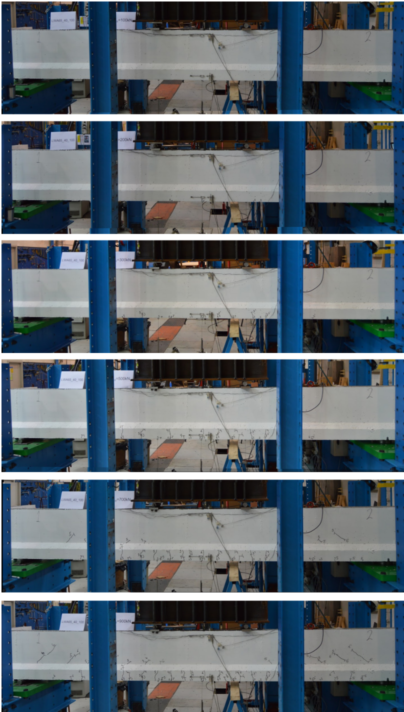
Figure B.6: Beam 6 - Load steps with drawn crack development.
