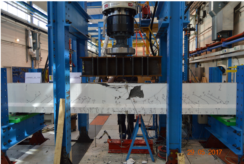
Figure 5.36: Beam 4 - Whole beam, failure
