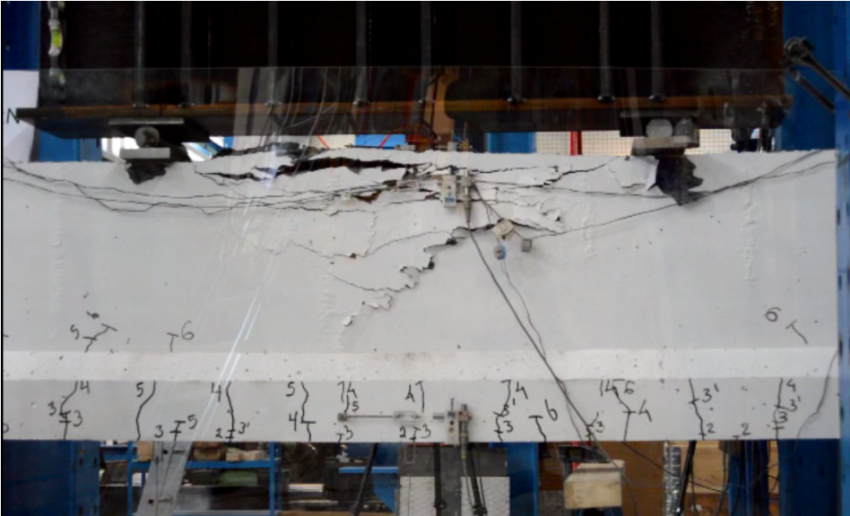
Figure 5.47: Beam 6 - Test zone, failure
