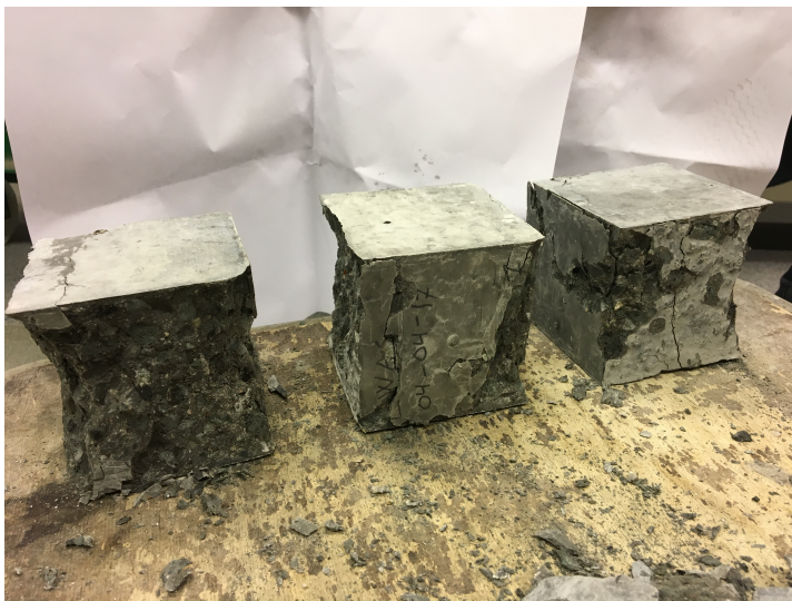
Figure 5.2: Failure of cubes in compression
