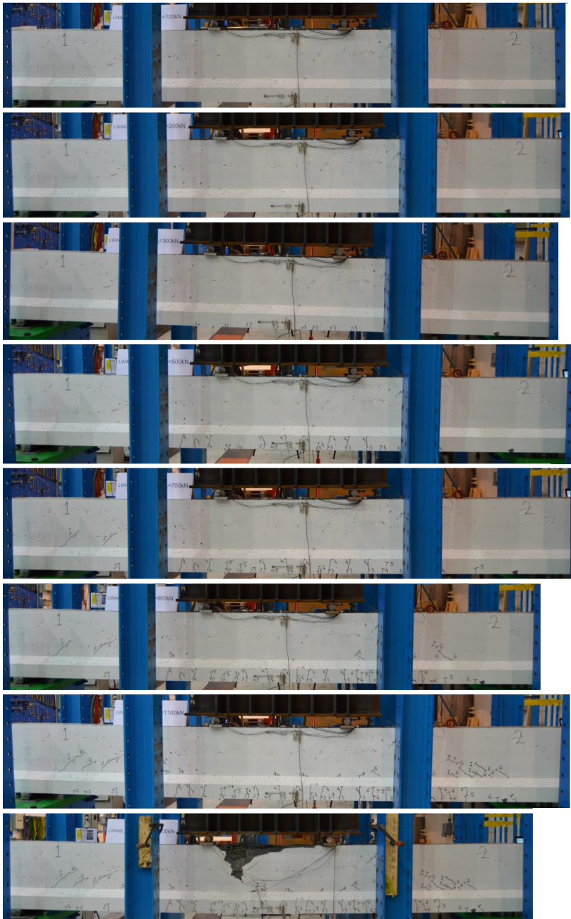
Figure B.3: Beam 2 - Load steps with drawn crack development.
