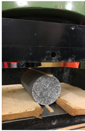
Figure 4.2: Cylinder in the Mohr Federhaff Losenhausen machine
