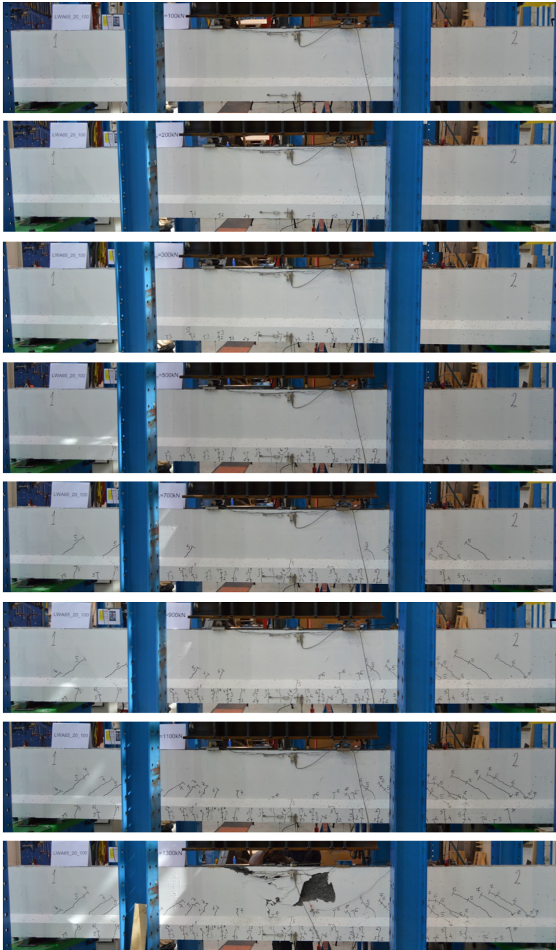
Figure B.5: Beam 4 - Load steps with drawn crack development.
