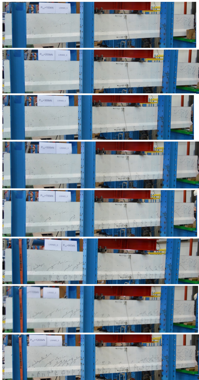
Figure B.1: Beam 1 - Setup 1 - Load steps with drawn crack development.
