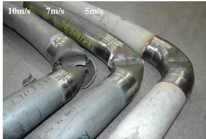
Fig. 12. Test samples with \sigma \approx 8 vol% after dynamic testing at various impact velocities (tests D3, D4 and D5).
