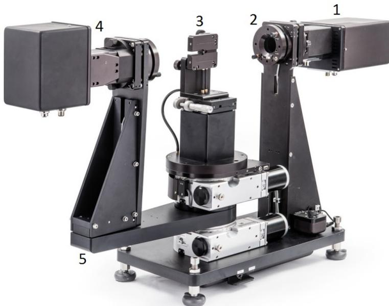
**Figure 4.1:** Experimental setup of the RC2 ellipsometer with 1) light source, 2) source optics, 3) vertical sample mount, 4) receiver optics and 5) goniometer arm for variable angle measurements. Figure adapted from [26].
