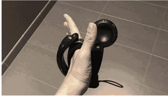
Figure 38: The upcoming Knuckles controller from HTC. The user can release the grip of the controller, and the controllers stay attached. Photo: [87]
