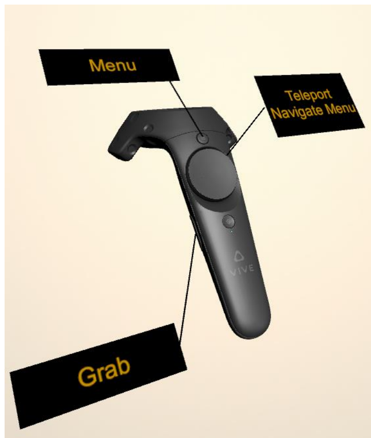
Figure 4 Room-scale controller tooltips. Each tooltip's line points directly to their respective button, guiding the user in the desired direction.
