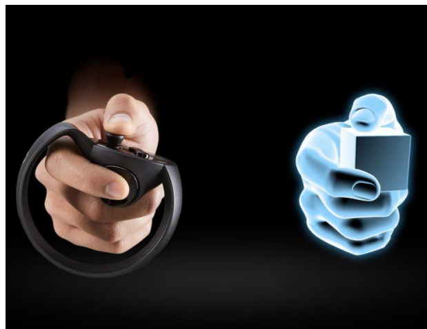
Figure 37: Oculus Touch being held by a user. This controller is easier to map to virtual, animated hands as the user's hands naturally rest inside the controller and all buttons have capacitive sensors. Photo: [88]
