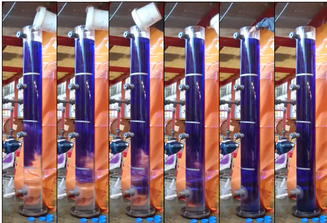
Figure 5.2 55 wt% potassium formate brine poured turbulent into the pipe after - 10 seconds - 12 seconds - 14 seconds - 16 seconds - 18 seconds - 20 seconds (from left to right).
