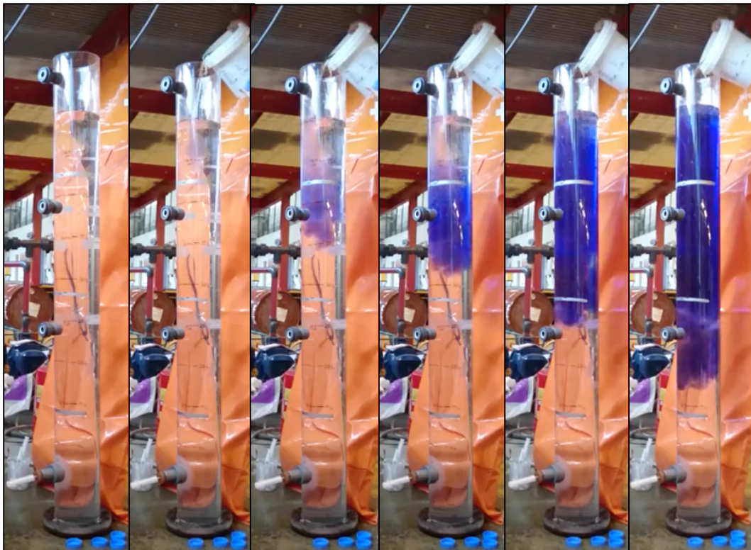
Figure 5.1 55 wt% potassium formate brine poured turbulent into the pipe after - 0 seconds - 0 seconds - 2 seconds - 4 seconds - 6 seconds - 8 seconds (from left to right).
