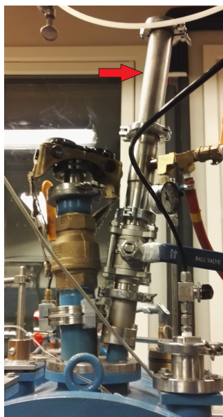
Figure 4.7 – Tube chamber for sampling. Red arrow indicates the insertion chamber.
