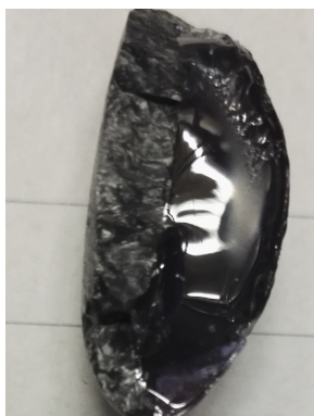
Figure 5.8 – Cross section of sample "MS1", showing the two phases.
