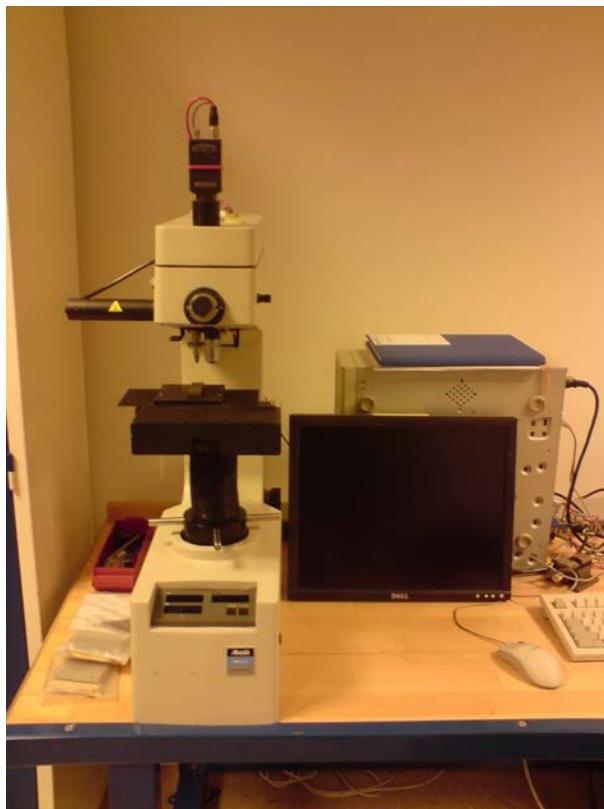
FIGURE 3.5. The Akashi hardness tester used for measuring the Vickers hardness.
