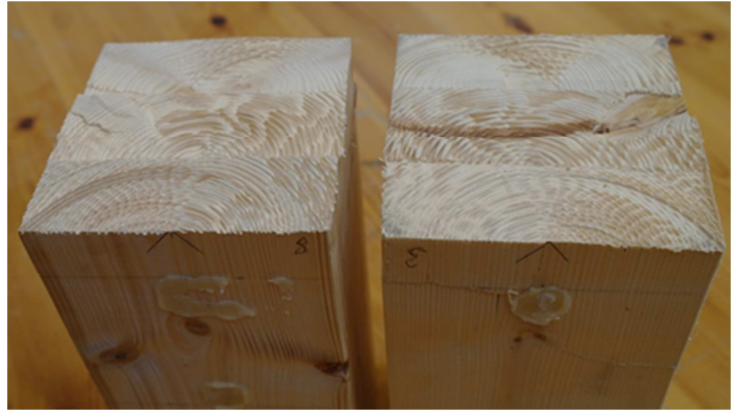
Figure 9: Deformation of the crushing zone during testing (left), and deformation pattern at the end faces after testing (right).
