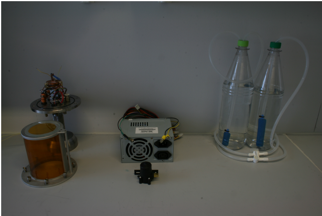
Figure 4.1: Picture of the entire test cell system. The sample cell can be seen to the left with the cap in front of the baseplate. The sample holder is mounted on the baseplate. In the middle the cooling/heating fluid pump can be seen with its 12 V power supply visible behind. To the right the bobble bottles of the gas humidifier is seen.
