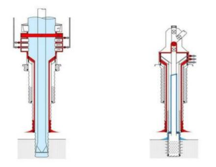
Figure 2: Two barrier envelopes where blue represents primary barrier and red represents secondary barrier(Anders et al., 2015)
