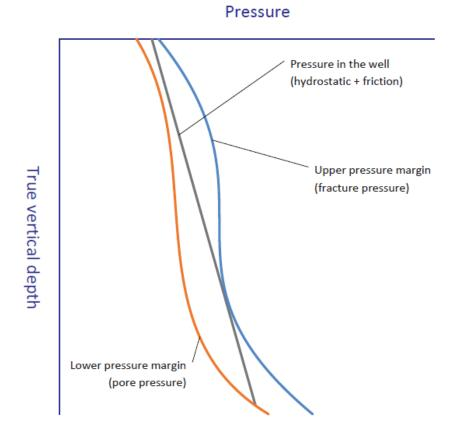
Figure 3: Pore pressure, Hydrostatic pressure and Fracture pressure(Hauge, 2013)
