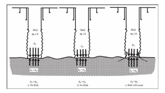
Figure 4: Drilling conditions, a. overbalanced, b. balanced and c. underbalanced.(Azar, 2007)
