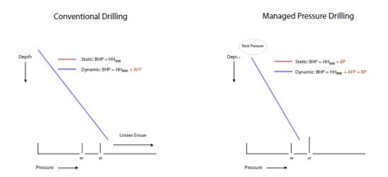
Figure 15: Differences between conventional and managed pressure drilling(Hilts, 2013).
