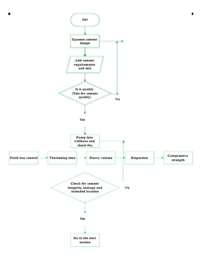
Figure 22: An example of steps or procedures for slurry design and pumping advisory program
