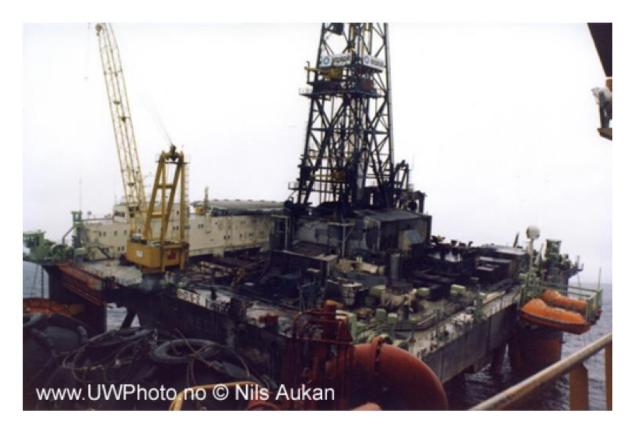
Figure 18:West Vanguard when the blowout broke; the main deck was damaged
