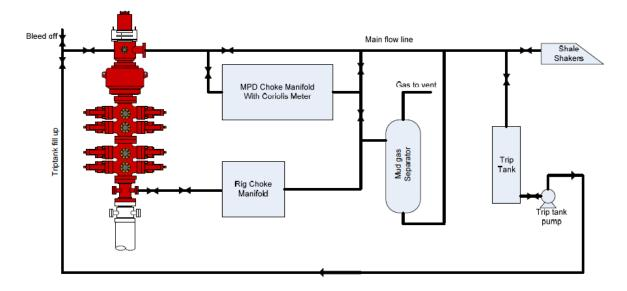
Figure 14: Managed pressure drilling setup in a closed wellbore(Nas, 2011)
