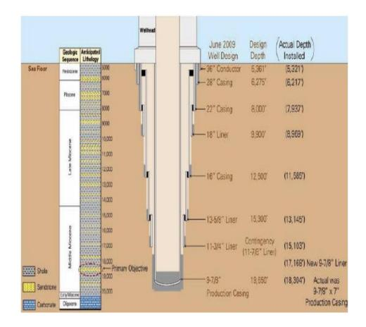
Figure 17: Geology and original design of Macondo well(Deepwater Horizon Study Group, 2011)
