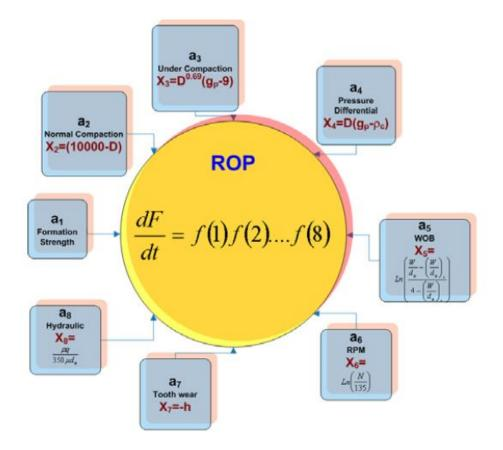
Figure 11: General rate of penetration equation (T. Eren & Ozbayoglu, 2011)
