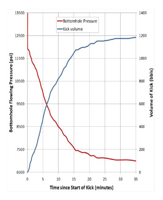
Figure 5: Relationship between bottom hole pressure and kick volume with time (Willson, 2012)
