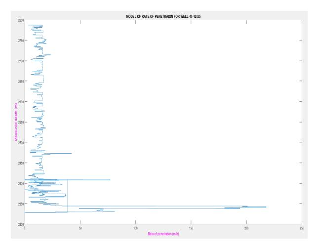
Figure 21: Rate of penetration variation with respect to measure depth
