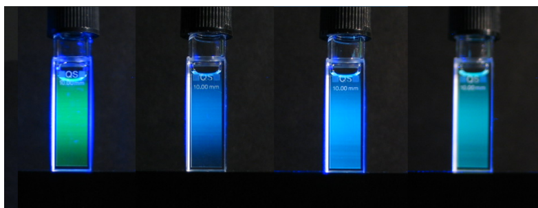
Figure 5.1: Picture of the fluorescence emission of Fluorescein, C110, C314 and C334, respectively. The samples show different emission colors in the blue-green region.
