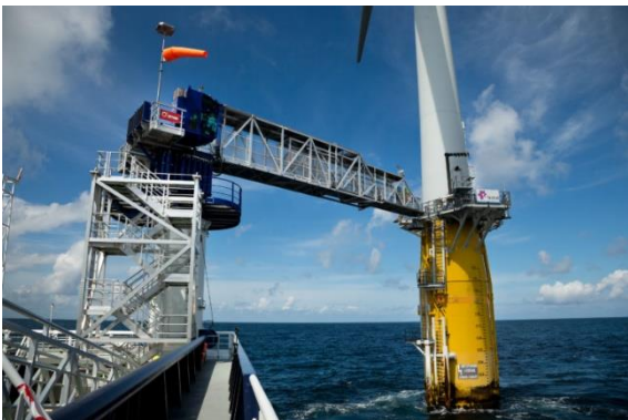
Fig. 1 Gangway transferring operation [3]
