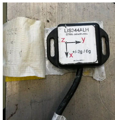
Figure 5.2: Accelerometer 1 attached to the shaking table.
