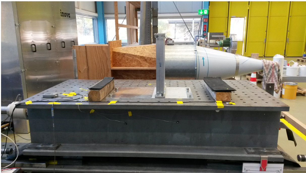
Figure 4.6: Picture of shaking table and test specimen. Notice the two pairs of optical markers on the side of the shaking table and on the test specimen. See figures 4.1 and 4.2 for further descriptions.
