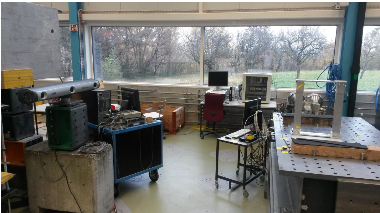
Figure 4.7: Overview picture of laboratory set up. The NDI optical sensor is seen to the left, the shaking table and the test specimen to the right. The three PCs are seen in the background. See figures 4.1 and 4.2 for further descriptions.
