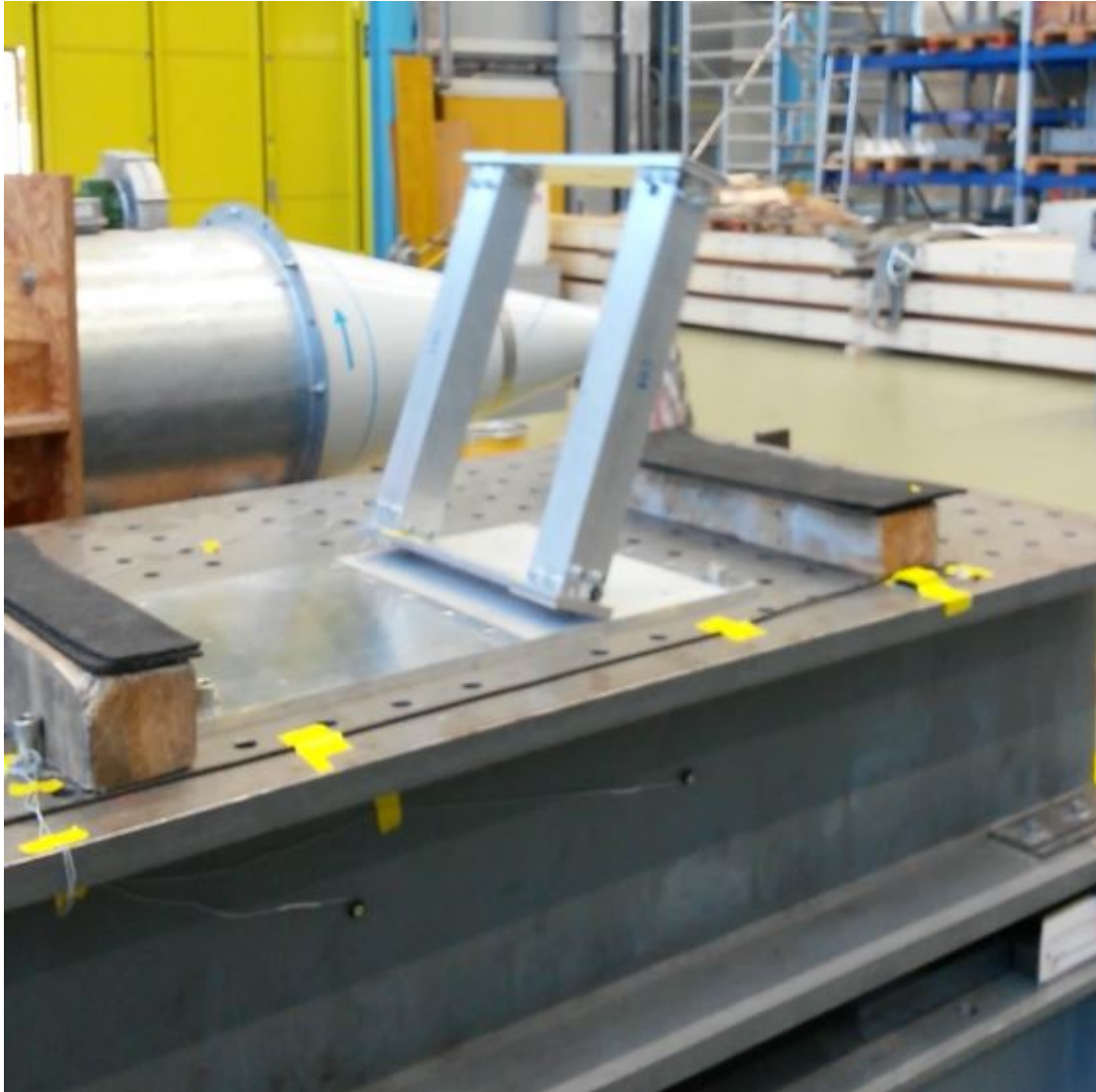
Figure 4.9: Rocking test specimen before overturning. Overturning lead to impacts that slightly influences the measured accelerations. The impacts lead additionally to that the bolts connecting the wedges and the columns become looser and must be re-tightened. See figures 4.1 and 4.2 for further descriptions.
