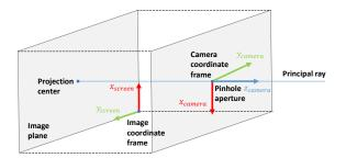
Fig. 1. Coordinate frames in the pinhole camera model.
