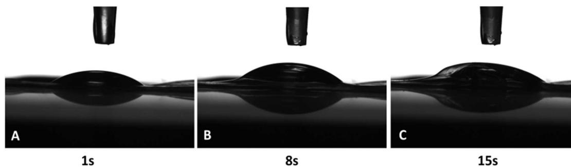
Figure 7 – Time evolution of a contact angle experiment performed depositing a 3D3M droplet on an Aquivion sample immersed for 24h in the 3D3M mixture at 60 °C.
