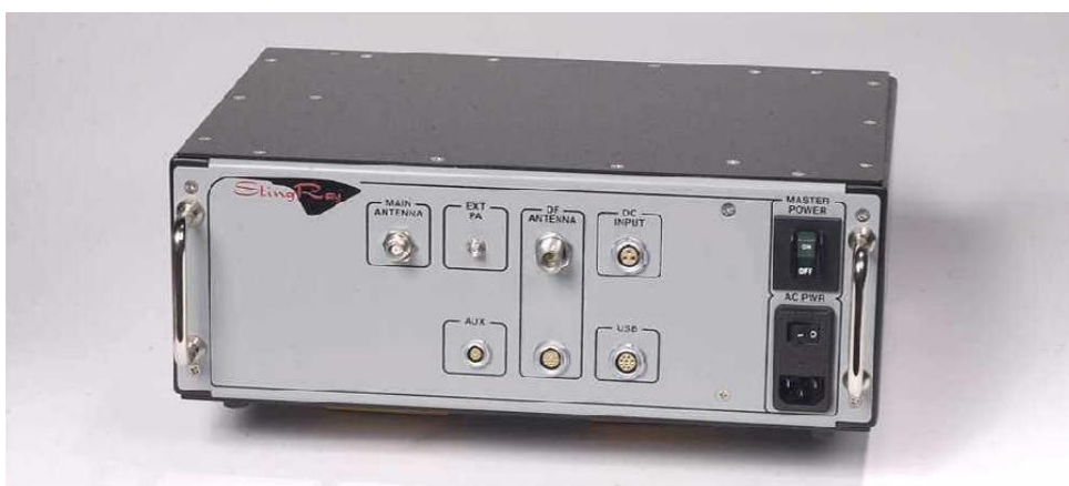
Figure 3.1: Harris Corporation’s first IMSI Catcher, the StingRay. Source: [Rya].
