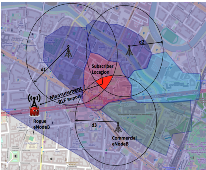
Figure 5.5: Locating a subscriber using the trilateration procedure. The solid red area indicates the location of the subscriber. Source: [SBA + 15].
