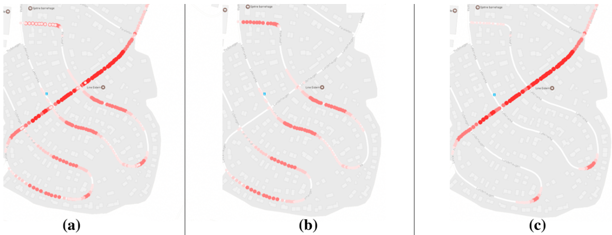
Fig. 19. Shows the results of applying different filtering to the data. (a) shows glare for both morning and evening rush hour. (b) shows only data for morning glare, whereas (c) shows evening glare.
