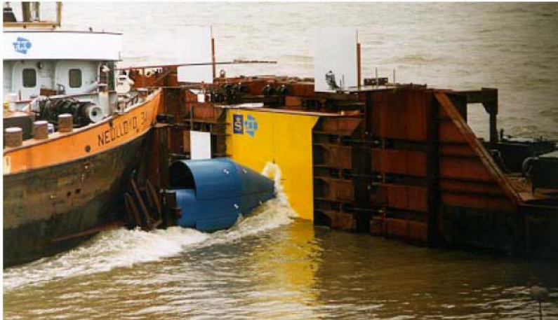
Figure 2-11. Full scale ship collision experiments in the Netherlands (Wevers et al., 1999)
