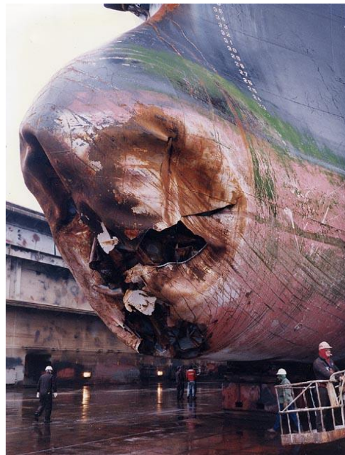
Figure 1-4. The damaged ship bow after OVERSEAS OHIO collided with an iceberg
