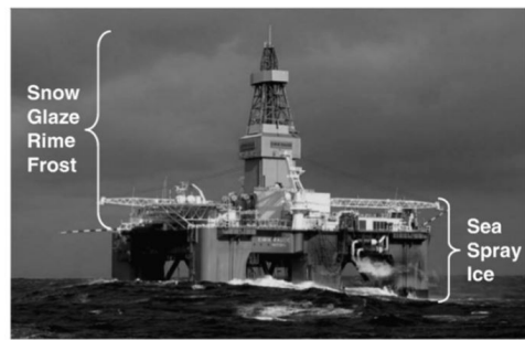
(b) Potential ice accretion areas, by ice type, on the Ocean Rig semisubmersible Erik Raude ([21]), [23]
