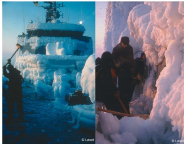
Figure 1.1: Icing on KV Nordkapp on the 27th of February 1987, Barents Sea. Left picture show the fore-ship and the wheel house, right picture show the starboard walkway and railings [24].
