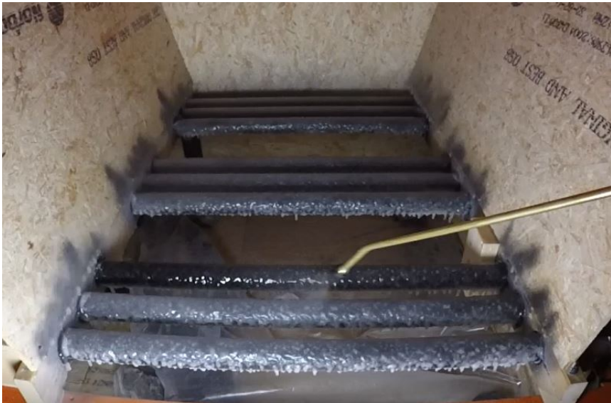
Figure 4.11: Icing - Manually application of the water spray.
