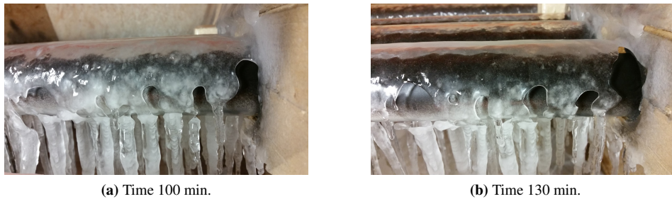
Figure 5.20: Picture showing the insulating layer of air between the pipe surface and the ice.
