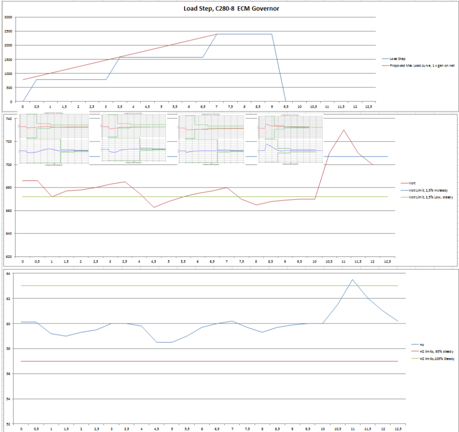
Figure 3-30, Sequent load steps in a row to try to illustrate engine capability
