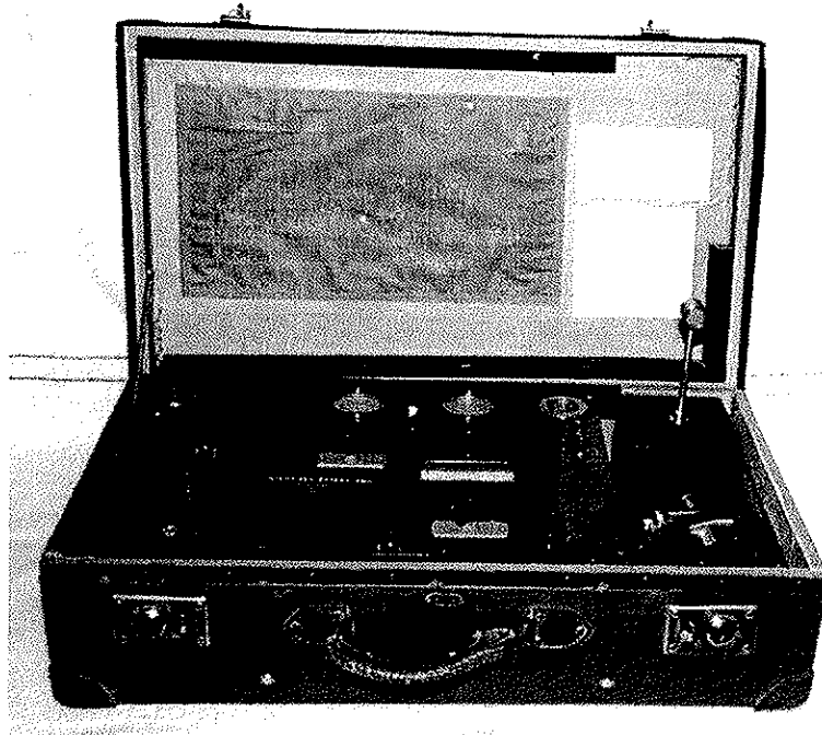
Fig. 4.8: Reverberation measurement apparatus built by Vebjørn Tandberg around 1931. One copy was made for NRK, the present one in the photo was kept at NTH's physics department (Photo: Roland Wittje).
