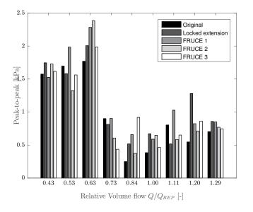
Figure 5. Peak-to-peak values for a 99% confidence interval for the lower measuring plane of the Francis model draft tube
