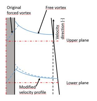
Figure 6. Ideal tangential velocity profiles at upper an lower measuring plane with FRUCE. The ideal velocity profile is shown with a dashed line in the lower plane and the modified velocity profile is shown with a solid line.
