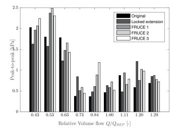
Figure 4. Peak-to-peak values for a 99% confidence interval for the upper measuring plane of the Francis model draft tube
