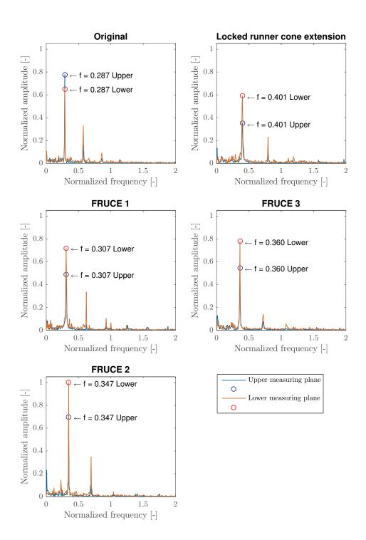
Figure 7. Frequency analysis for  $0.63Q/Q_{BEP}$  with upper and lower measuring plane
