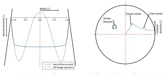
(a) Axial velocity profile (b) Tangential velocity profile with vortex filament
