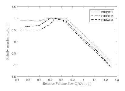
**Figure 3.** FRUCE rotation as a function of flow rate. The relative speed is given by the FRUCE rotational speed,  $n_s$ , and the runner speed,  $n_t$ .
