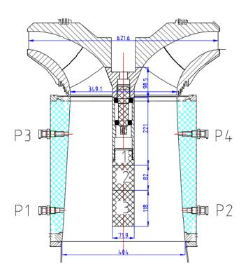
Figure 2. Freely rotating runner cone extension with the different lengths; FRUCE  $1 = 0.62D_2$ , FRUCE  $2 = 0.86D_2$  and FRUCE  $3 = 1.20D_2.$ The location of pressure sensors can be seen on the draft tube wall. The dimension in the drawing is given in millimeters
