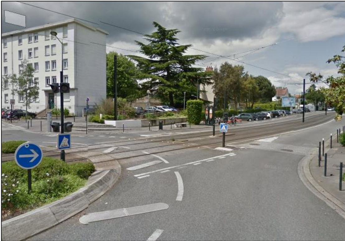
Figure 6: Dedicated, centred tram lanes through a roundabout in Nantes, France. [Source: Google Maps – street view]
