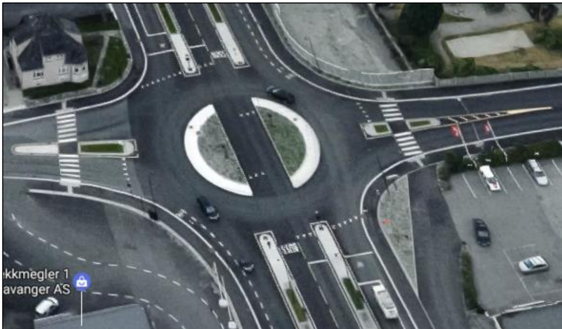
Figure 5: Dedicated, centred bus lanes through a roundabout in Hillevågsveien, Stavanger. [Source: Google Maps – street view]
