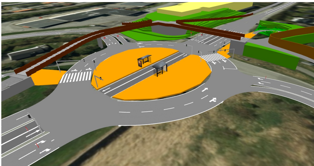
Figure 4: Concept 2 - Signalised roundabout with bus stop in the centre island in 3D seen from northeast
