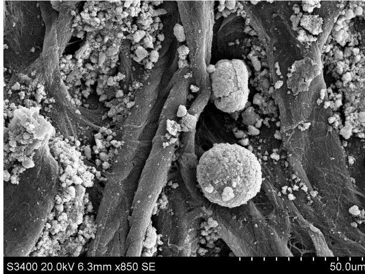
Figure 4.16: SEM image of a sample obtained directly from the process at Glencore. The background is fibers from the filter paper.
