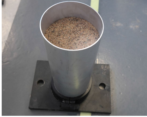
Figure 4: The aluminum tube used to contain the sand in the tests
