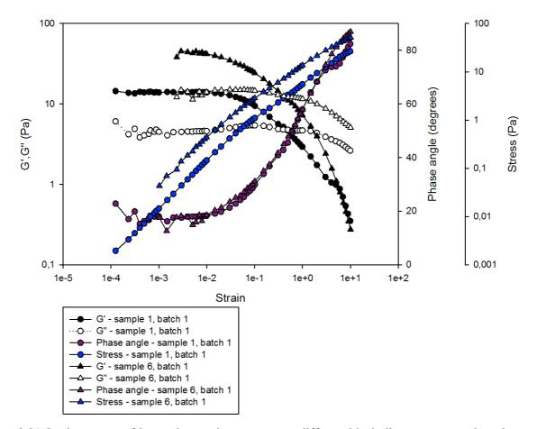
**Figure 3.31** Strain sweeps of increasing strains run on two different biosimilar mucus samples taken from mucus batch number one. Circles represent sample 1 and triangles represent sample 6. The fixed frequency of the sweeps were 1 Hertz, and the temperature 25 °C.
