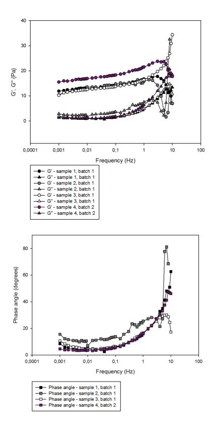
**Figure 3.28** Four replicate strain controlled frequency sweeps of different biosimilar mucus samples, in the frequency range 0.001-10 Hertz. The fixed strain for all the measurements was within the linear viscoelastic region, and the temperature was 25 °C. The moduli values are presented in the upper plot, and the phase angle values are presented in the lower plot.
