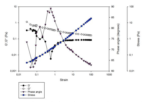
**Figure D.6** Stain sweep of a 10 % (w/v) Sigma mucin solution in the strain range 0.001-100. The temperature of the measurement were 37 °C, and the frequency 1 Hertz.
