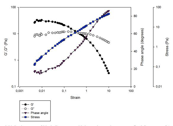
**Figure 3.30** Strain sweep of biosimilar mucus with increasing strains, run at a fixed frequency of 1 Hertz and a temperature of 25 °C.
