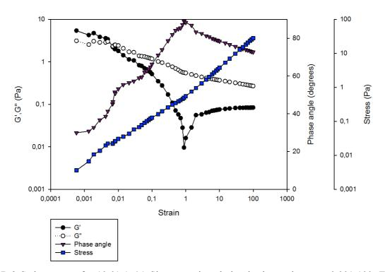
Figure D.3 Stain sweep of a 10 % (w/v) Sigma mucin solution in the strain range 0.001-100. The temperature of the measurement were 25 °C, and the frequency 1 Hertz.
