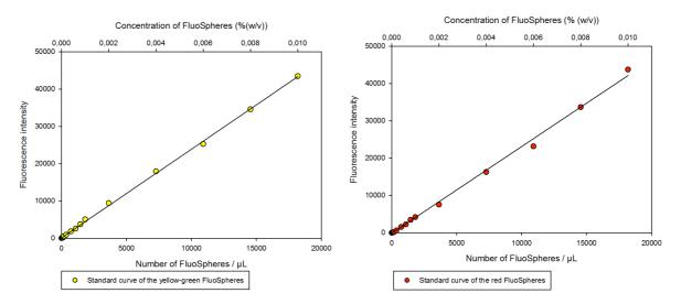
**Figure 3.17** Standard curves of the FluoSpheres® yellow-green (left) and red (right), made with average values of three replicates. The ex./em. wave-lengths of the measurements were 495/535 nm for the yellow-green particles, and 580/615 nm for the red particles. The volume of nanoparticle solution in each well was 100  $\mu$ L.
