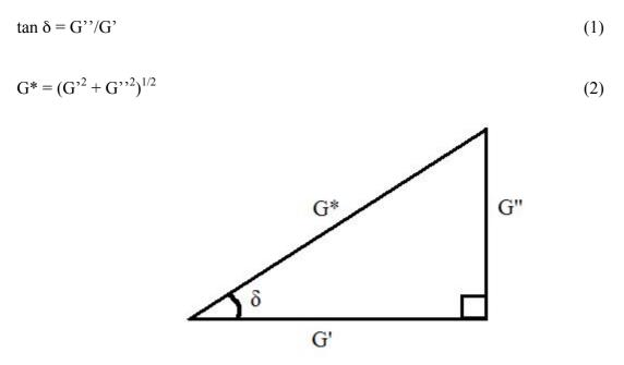
**Figure 1.7**. The relationship between the storage modulus (G'), the loss modulus (G''), the complex shear modulus (G\*) and the phase angle ( $\delta$ ). Modified from (Chaplin, 2012).
