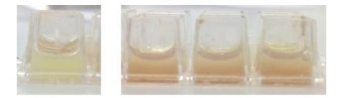
**Figure 3.8** Side view of glass chambers containing different 0.1% (w/v) nanoparticle solutions on top of 0.1 g biosimilar mucus (left) and 0.1 g PSIM (right). The pictures were captured straight after addition of nanoparticles.
