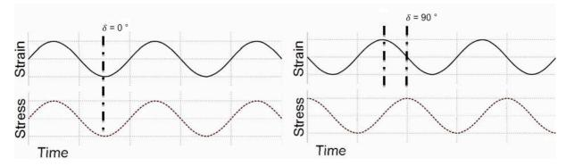
**Figure 1.6** The phase lag between the stress and strain waves of a perfectly elastic material (left) and a perfectly viscous material (right). A perfectly elastic solid will immediately respond to the stress, and the phase angle between the two waves is 0 °. A perfectly viscous material will have a strain wave that is 90 ° out of phase with the stress wave. A viscoelastic material will behave in between these two extremes. Modified from (Society of Plastics Engineers, 2012).
