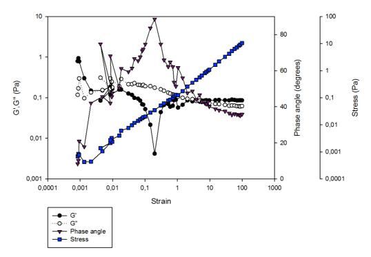
**Figure D.4** Stain sweep of a 5 % (w/v) Sigma mucin solution in the strain range 0.001-100. The temperature of the measurement were 37  $^{\circ}$ C, and the frequency 1 Hertz.
