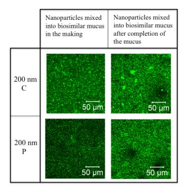
**Figure 3.5** Confocal images in the XY direction of 200 nm sized carboxylate-modified (C) and PEGylated (P) nanoparticles mixed in biosimilar mucus. In the images of the first column, the nanoparticles are added in biosimilar mucus in the making, and in the images of the second column the nanoparticles are added to biosimilar mucus already made.
