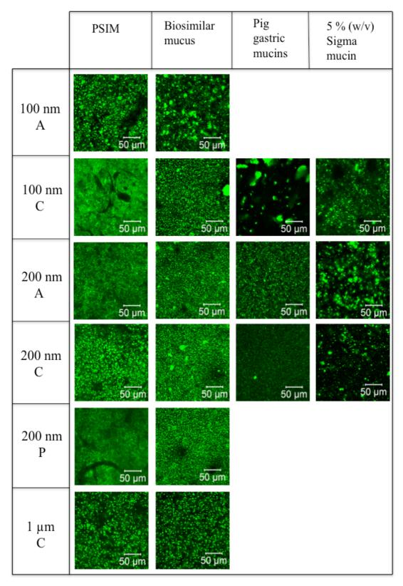
**Figure 3.1** XY confocal images captured of various types of fluorescent nanoparticles mixed into different mucous systems. The size and charge of the nanoparticles are indicated in the column to the left, were A = amine modified (+), C = carboxylate modified (-) and P = PEGylated (-).
