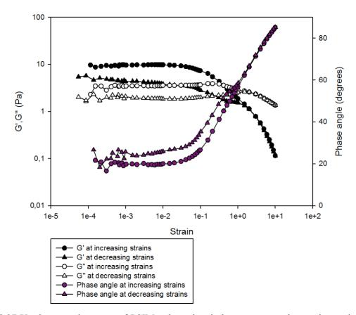
**Figure 3.27** Up-down strain sweep of PSIM, where the circles represent values at increasing strains and the triangles represent values at decreasing strains. The sweep was run at a frequency of 1 Hertz and at 25  $^{\circ}$ C.
