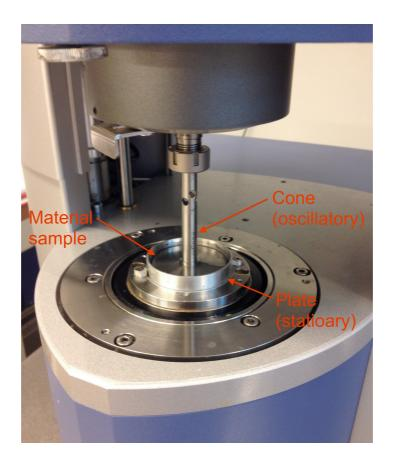
**Figure 1.5** The set-up of a rheometer. The material sample is put on the plate and the cone is lowered on top of it before the measurements starts.
