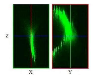
**Figure 3.12** XZ and YZ confocal images of 100  $\mu$ L 0.1 % 1  $\mu$ m carboxylate-modified nanoparticles put on top of 0.10 g 5 % (W/V) pig gastric mucin matrix. The nanoparticles were found in channels and holes in the matrix near the bottom of the glass chamber.
