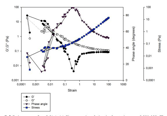
**Figure D.5** Stain sweep of an 8 % (w/v) Sigma mucin solution in the strain range 0.001-100. The temperature of the measurement were 37 °C, and the frequency 1 Hertz.
