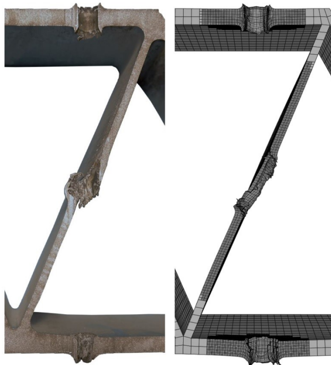
Figure 24: Pictures of an experiment and a simulation of a sand-filled panel to show the qualitative similarities. Left: experiment ( v_i = 910.5 m/s and v_r = 485.4 m/s). Right: simulation ( v_i = 900.0 m/s and v_r = 431.0 m/s).
