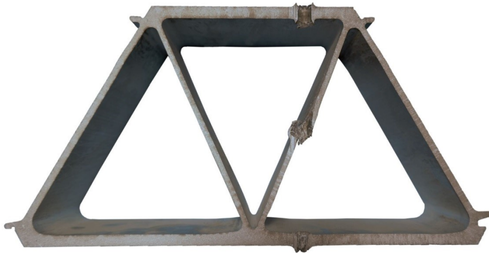
Figure 8: Cross section of an AA6005-T6 panel that was struck when filled with B95 sand: v_i = 910.5 m/s and v_r = 485.4 m/s.
